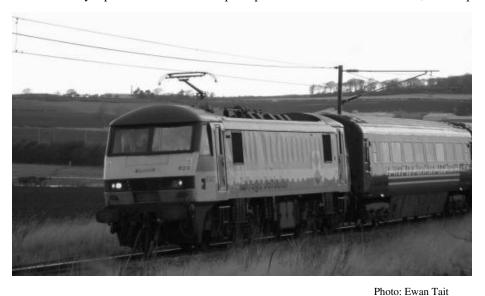
the North Berwick branch service, each comprising a Class 90 locomotive, 4 ex-Virgin West Coast Mk III coaches and a DVT. The latter is a Driving Van Trailer in which the driver sits when the loco is in push mode and is the same as the GNER's East Coast Main Line 225 sets. This means that turnround facilites at North Berwick are not required. This setup was tested on December 21st for lineside clearance on the branch, as seen in the above photograph.
